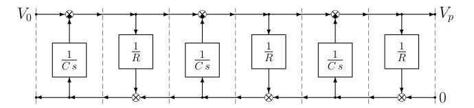
One can easily verify that applying the Mason's formula to this block scheme one obtains the same transfer function G(s) obtained applying the Mason's formula to the previous block scheme.
