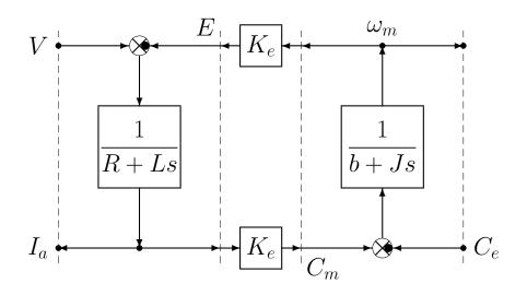
• The output variable  $\omega_m(s)$  can be expressed as a function of the input variables V(s) and  $C_e(s)$  as follows:
