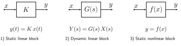
• In the block diagrams, the individual oriented elements are connected to each other by "branch points" and "summation points":
