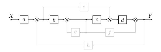
• A <u>ring</u> is a closed path. The <u>coefficient</u> A of the ring is the product of the gains of the branches that compose the ring. Example: the coefficient  $A_2$  of the ring highlighted in the following figure is  $A_2 = bcdh$ .
