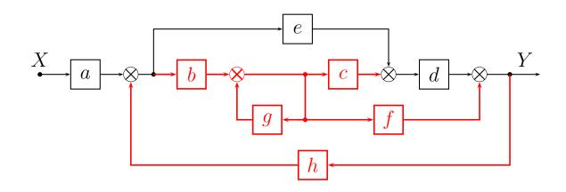
• For the considered system, the  $\Delta_i$  determinants of the partial block schemes associated with the  $P_i$  paths are as follows:
