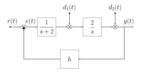
• Calculate the steady-state value of the variable e(t) in the presence of the following signals: r(t) = t,  $d_1(t) = 1$  and  $d_2(t) = 1$ .
