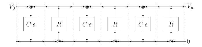
The transfer function G(s) which links the input  $V_0(s)$  to the output  $V_p(s)$  can be easily obtained using the Mason's formula:
