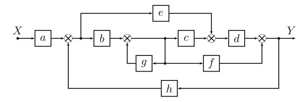
• A <u>path</u> is a sequence of adjacent branches and nodes without rings in which each element is crossed only once. The <u>coefficient</u> P of the path is the product of the gains of the branches that compose the path. Example: the coefficient  $P_1$  of the path highlighted in the following figure is  $P_1 = abcd$ .
